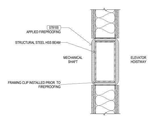
8 ELEVATOR - SHAFT WALL AT HSS BEAM IN CAVITY A502 1 1/2" = 1'-0"
