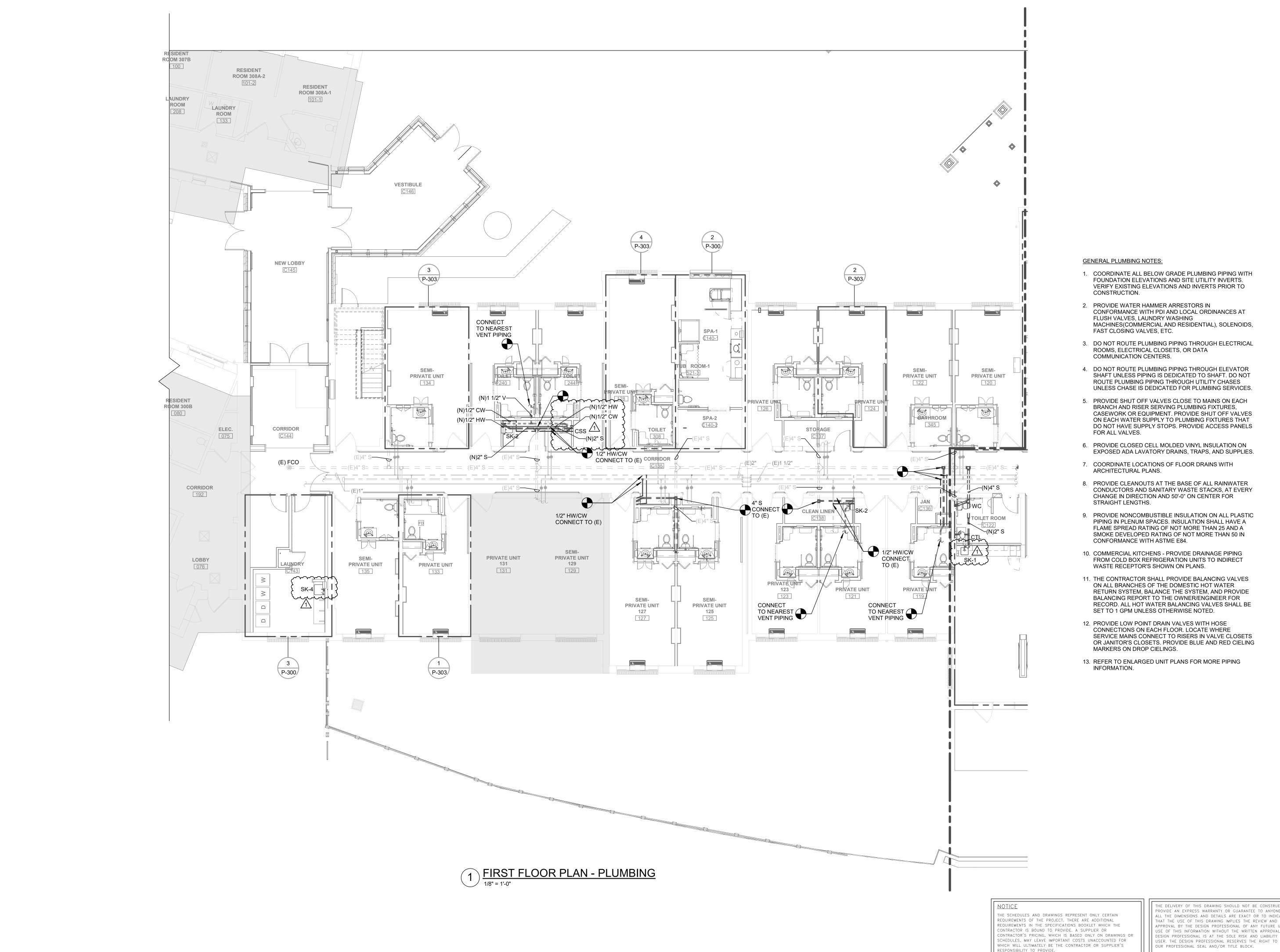
1. COORDINATE ALL BELOW GRADE PLUMBING PIPING WITH FOUNDATION ELEVATIONS AND SITE UTILITY INVERTS. VERIFY EXISTING ELEVATIONS AND INVERTS PRIOR TO
