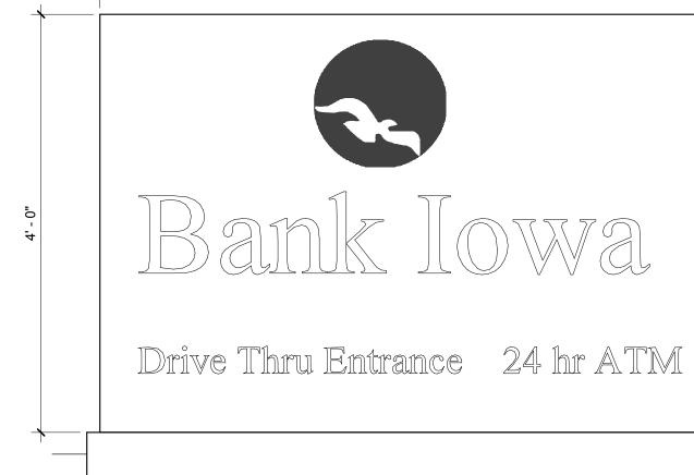
MONUMENT SIGN 3D BOX SIGN; 10" DEEP FACE: WHITE ACRYLIC SIDES AND EDGE TRIM: PAINTED BLACK ALUMINUM LIGHTING: INTERNALLY LIT MOUNT: BASE MOUNTED; CONCRETE FOOTING BY CONTRACTOR; COORDINATE ELECTRICAL CONNECTION WITH CIVIL AN .EPS OR .DXF FILE WILL BE PROVIDED FOR THIS GRAPHIC
