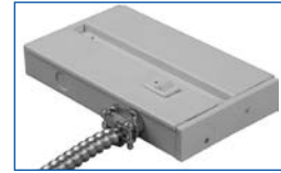
Switch Box • 120VAC input • White Finish • (6) .25" electrical knockouts • (1) output for flexible connector • Suitable for dry locations CAT. # CL-138528WH (Switch Box) CAT. # CL-138529WH (Switch Box w/ 3-way rocker switch integral occupancy sensor)
